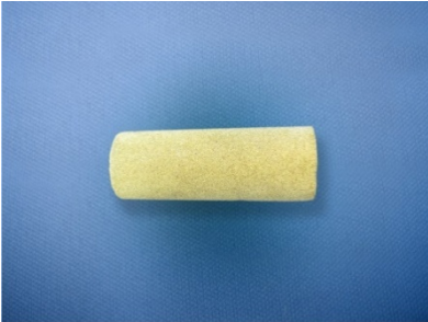
Fig. 3 – Sintered bronze tip
