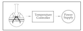
Once the mantle has been properly setup, plug the mantle into an acceptable temperature controller. Use a variable transformer, manual control, or automatic controller to prevent overheating.
