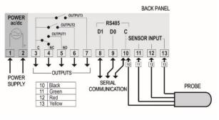
Figure 2 – Electrical connections
